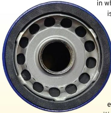
The idea for the change is for oil pressure to build more quickly at engine startup and allow for greater oil flow during hard acceleration and high RPM events, which will better protect critical engine bearing surfaces from wear. There will be no changes to the overall height or diameter of the filter.
