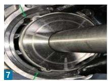
Step 7 - Install the Disconnect Rotary Cam onto the shaft, with the engagement teeth facing away from the housing. Install the Disconnect Linear Cam back onto the shaft with teeth facing the Rotary Cam and housing. Install the Worm Gear using a flat-bladed screwdriver, rotating until you hear an audible click.
