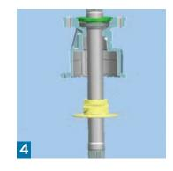
Step 4 – Remove the Power Transfer Disconnect Rotary and Linear Cams from the Extension Housing, shaking the assembly to get the cams to slide down the intermediate shaft. Check the Linear Cam for signs of abrasion or scratches and replace if necessary.
