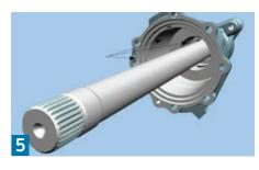
Step 5 — Inspect the Extension Housing for internal damage, and then clean its parts thoroughly — paying close attention to the Rotary Cam Bore and Worm Gear Bore, along with the bearing at the bottom of the latter. Dry the components using compressed air to remove any remaining solvent.
